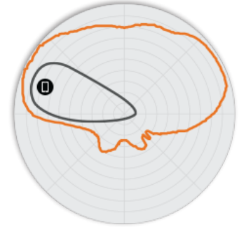
Figure 5. R720 5GHz Elevation Antenna Patterns
